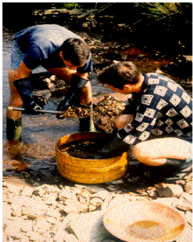
Figure 13. Wet sieving of a stream sediment sample in the UK (Photo: Fiona Fordyce, BGS from Salminen and Tarvainen et al. 1998, Fig. 7, p.21).
