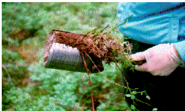
Figure 15. Humus sampling in Finland using cylindrical sampler, and the final humus sample. (Photographs: Timo Tarvainen, GTK).
